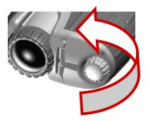
Open the door to install batteries.
