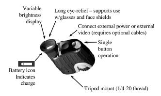
Model & serial number behind the external connections plug
