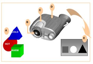
Infrared energy is emitted proportionally to the temperature of an object A. The warmer the object, the more energy it emits. The infrared energy from the objects is focused by the optics B, onto an infrared detector C. The information from the infrared detector is passed to electronics D for image processing. The signal processing circuitry translates the infrared detector data into an image E that can be viewed on the built-in video monitor.
